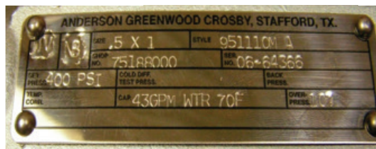
FIGURE 3-12 Typical ASME Section VIII Nameplate
